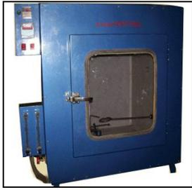
The **ASIAN Toxicity Chamber** is to consist of an airtight enclosure of about 1m<sup>3</sup> volume lined with opaque plastic sheeting having a hinged, fitted with a transparent plastic panel.
